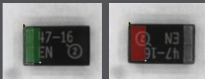
Capacitor oriented correctly
